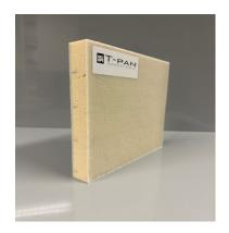
Sandwich panel with GRP skins with gelcoat suitable to the contact with foodstuffs and protection film, (on demand it is possible to deliver panels with different colours of GRP skins). Core: PVC foam.
