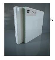
Sandwich panel with GRP skins with gelcoat suitable to the contact with foodstuffs and protection film, (on demand it possible to deliver panels with different colours of GRP skins). Core: expanded recycled PET or virgin.
